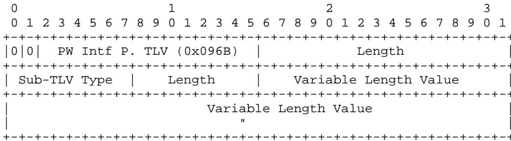
A more detailed description of this field can be found in Section 6.4 ("InterfaceParameter Sub-TLV").
