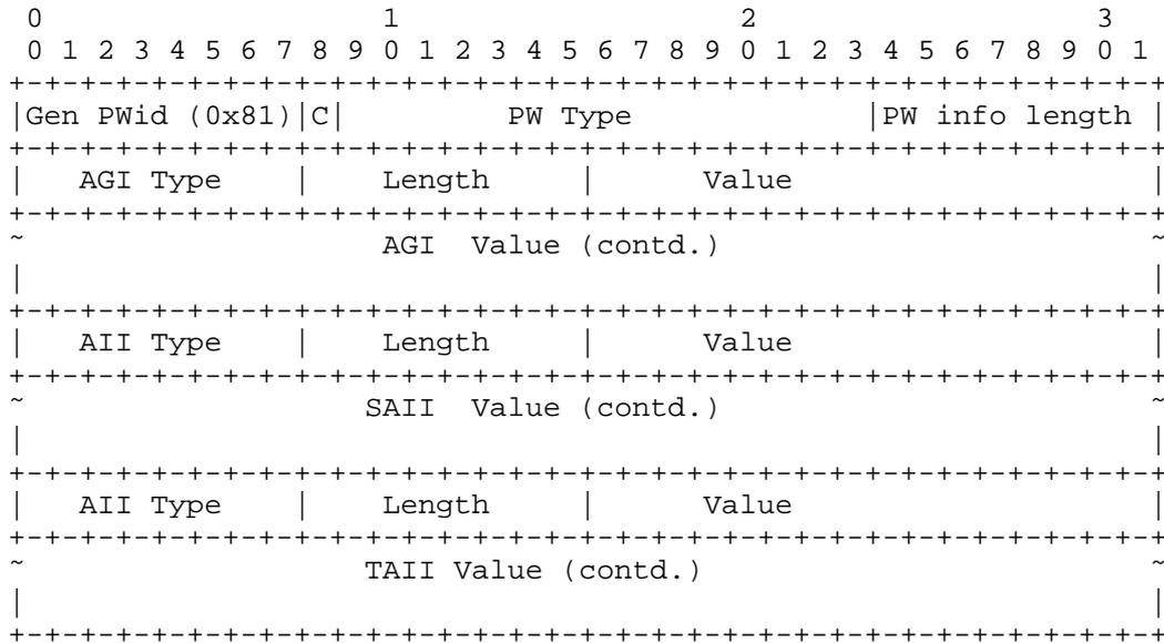
This document does not specify the AII and AGI type field values; specification of the type field values to be used for a particular application is part of the specification of that application. IANA has assigned these values using the method defined in [RFC4446].
