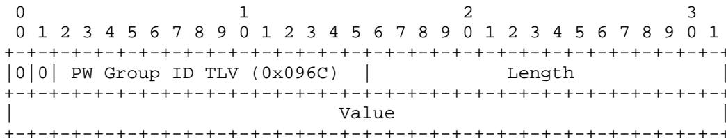
The PW Group ID is an arbitrary 32-bit value that represents an arbitrary group of PWs. It is used to create group PWs; for example, a PW Group ID can be used as a port index and assigned to all PWs that lead to that port. Use of the PW Group ID enables a PE to send "wildcard" label withdrawals, or "wildcard" status Notification messages, to remote PEs upon physical port failure.
