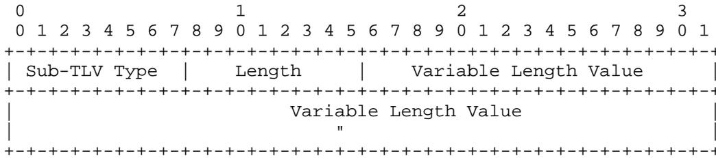
The Length field is defined as the length of the interface parameter including the Sub-TLV Type and Length field itself. Processing of the interface parameters should continue when unknown interface parameters are encountered, and they MUST be silently ignored.
