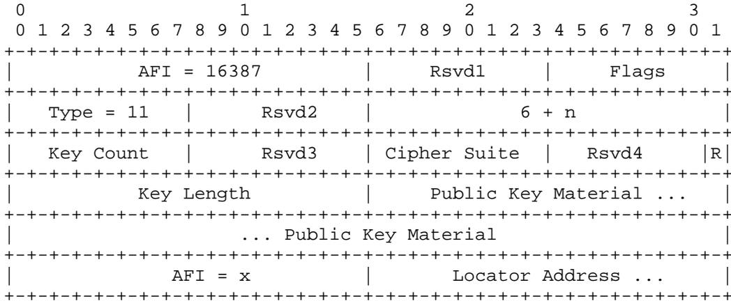
Cipher Suite Field Contains DH Key Exchange and Cipher/Hash Functions
