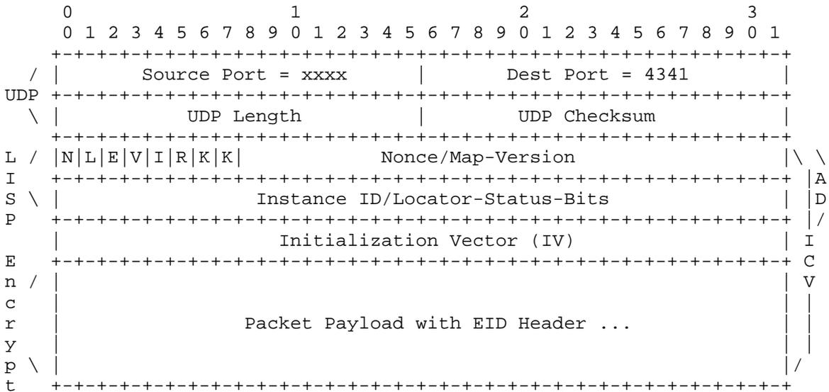
K-bits Indicate When a Packet Is Encrypted and Which Key Is Used
