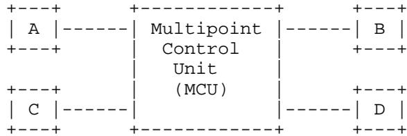
Figure 18: Point to Multipoint Using a Video-Switching MCU
