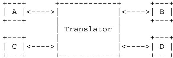
Figure 12: RTP Translator (Relay) with Only Unicast Paths
