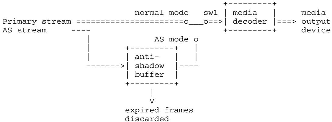
Figure 2: Anti-Shadow RTP Receiver
