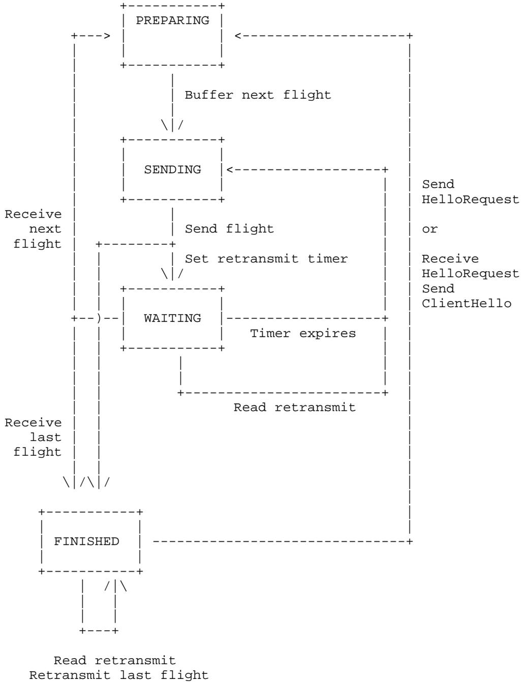
Figure 3. DTLS Timeout and Retransmission State Machine
