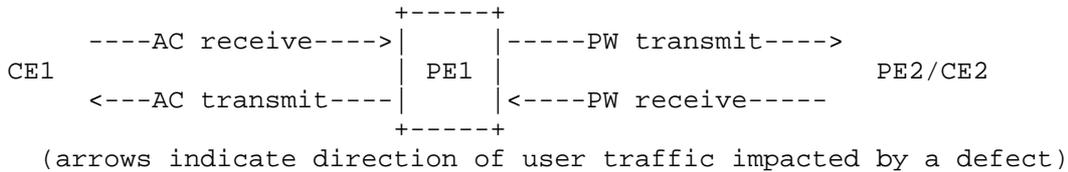
Figure 2: Receive and Transmit Defect States
