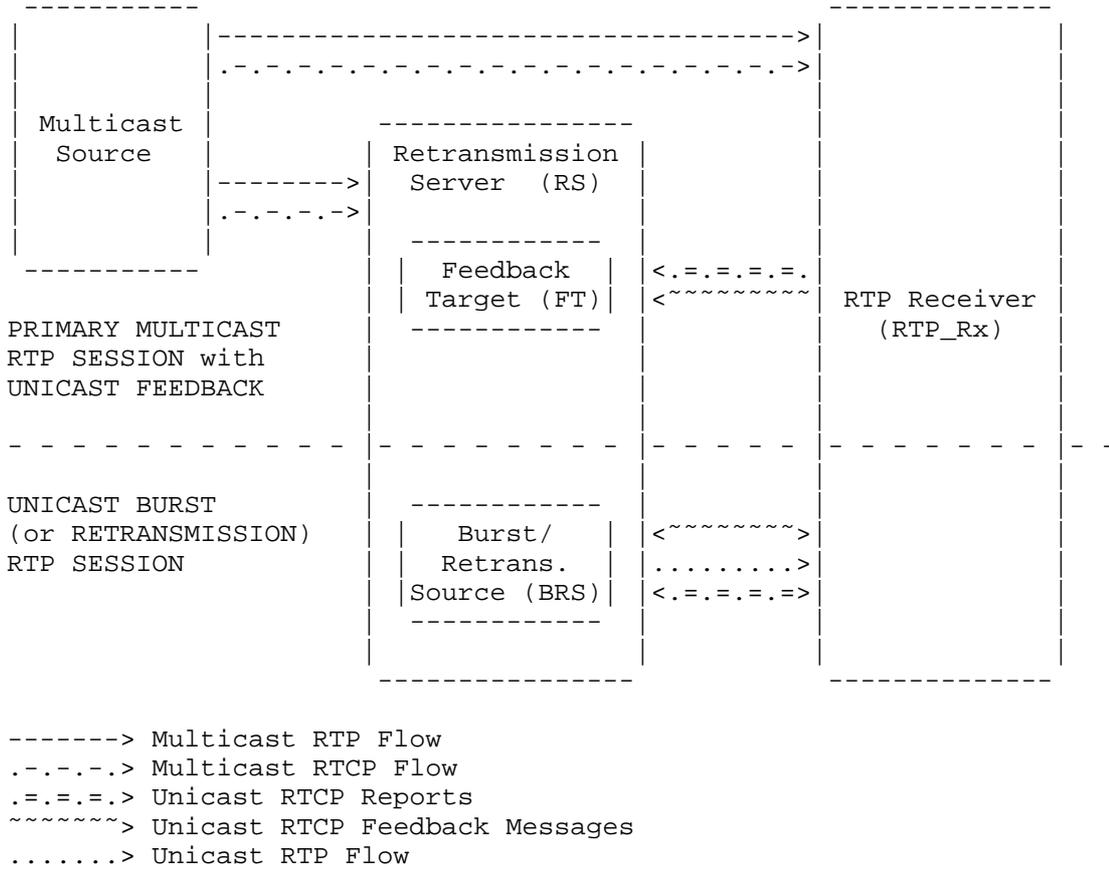
Figure 2: Flow Diagram for Unicast-Based Rapid Acquisition
