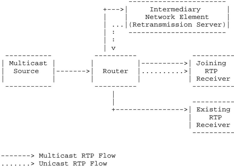
Figure 1: Rapid Acquisition through an Intermediary Network Element
