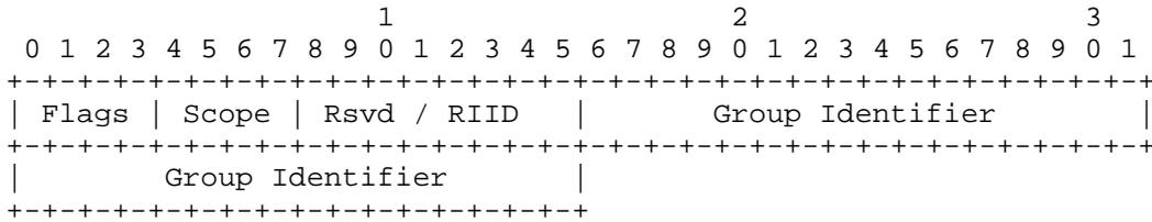
Figure 10: DAM = 00. Unicast-Prefix-based IPv6 Multicast Address Compression
