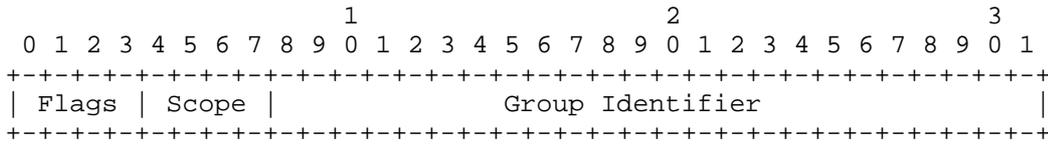
Figure 8: DAM = 10. 32-bit Compressed Multicast Address (ffFS::00GG:GGGG)
