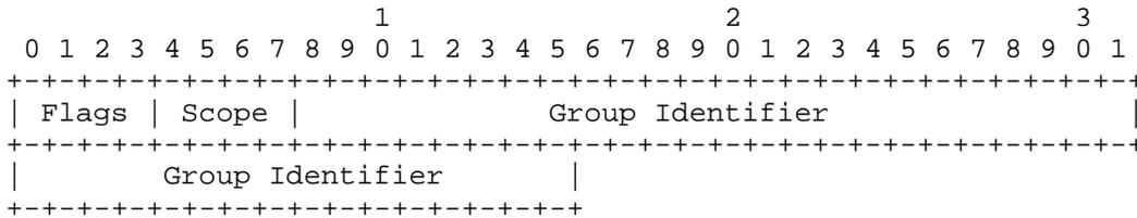
Figure 7: DAM = 01. 48-bit Compressed Multicast Address (ffFS::00GG:GGGG:GGGG)
