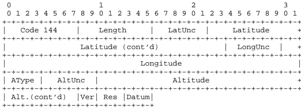
Code: 8 bits. The code for the DHCPv4 GeoLoc Option (144).
