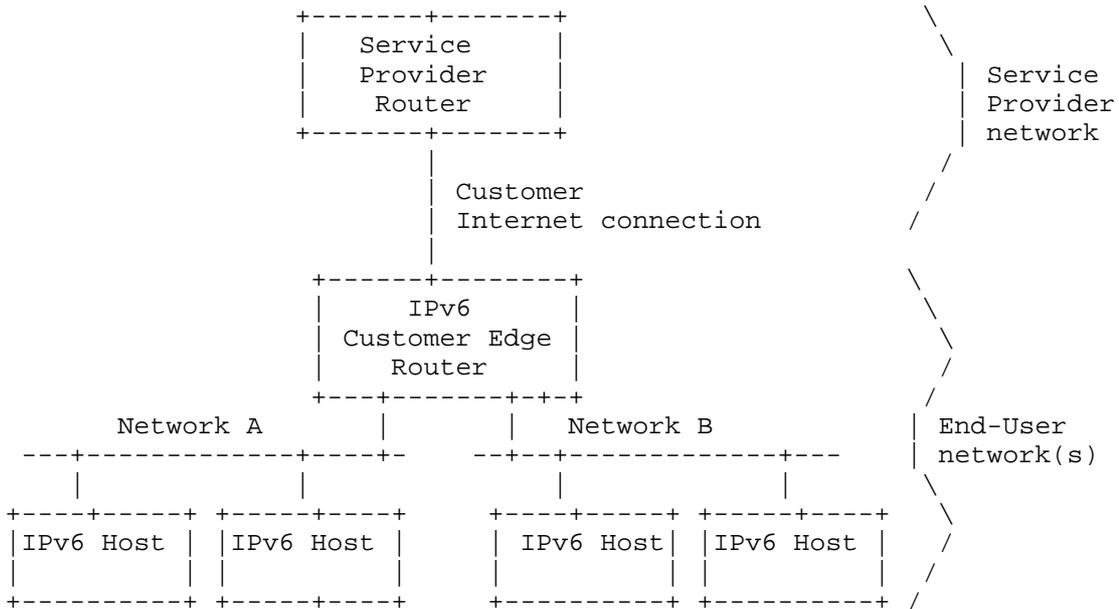
Figure 1: An Example of a Typical End-User Network
