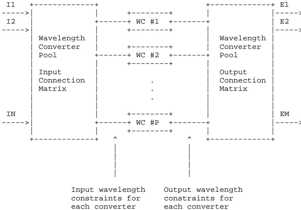
Figure 3. Schematic Diagram of Wavelength Converter Pool Model
