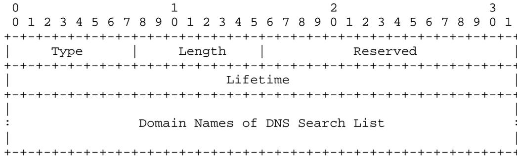
Figure 2: DNS Search List (DNSSSL) Option Format
