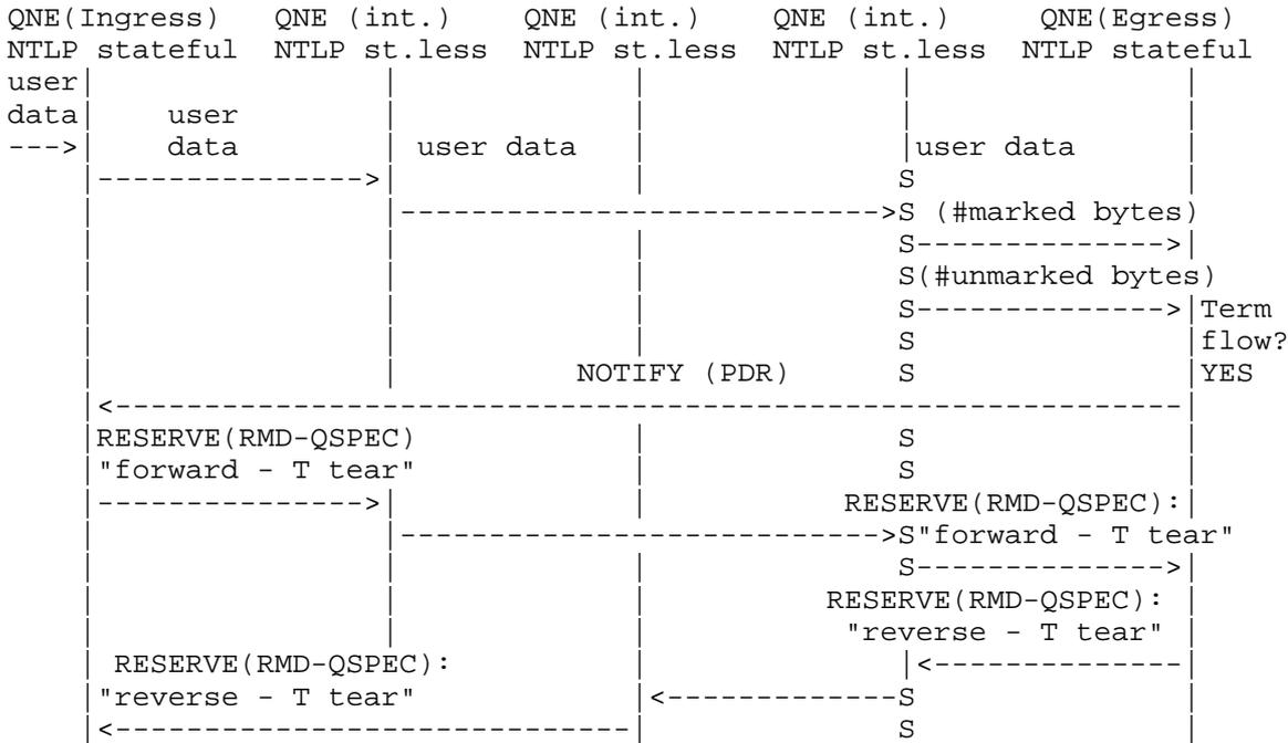
Figure 20: Intra-domain RMD severe congestion handling for bidirectional reservation (congestion on path QNE(Ingress) towards QNE(Egress))
