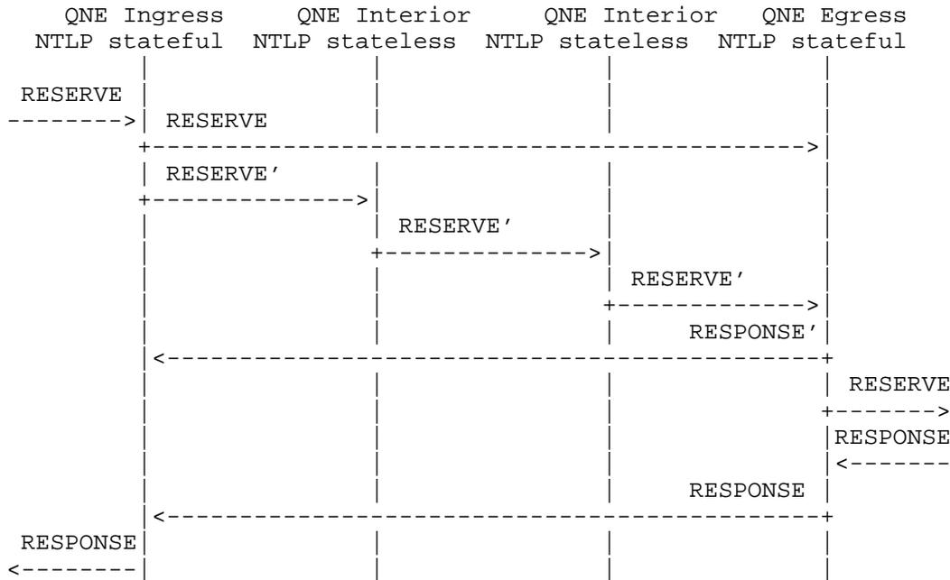
Figure 3: Sender-initiated reservation with reduced-state Interior nodes
