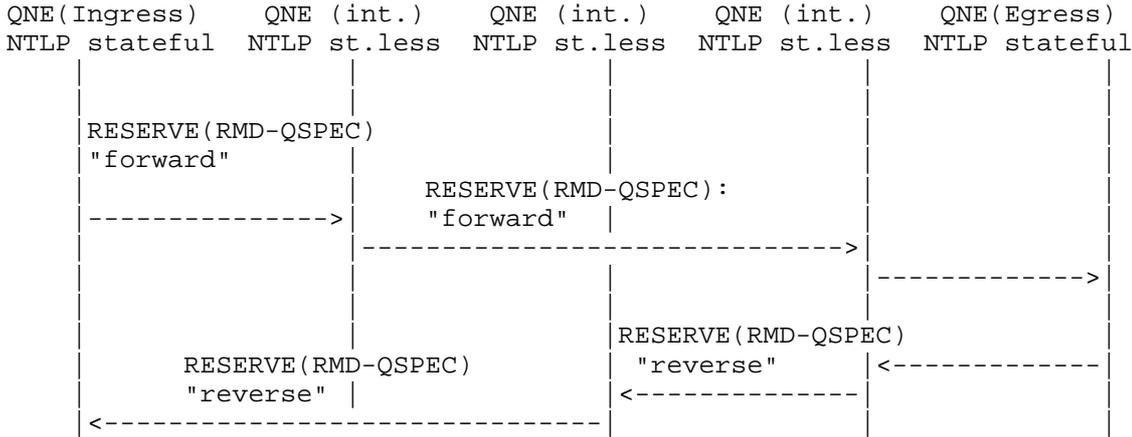
Figure 17: Intra-domain signaling operation for successful bidirectional reservation
