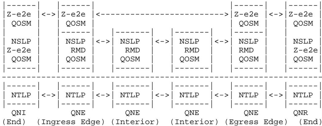
Figure 29. Example of initiator and local domain QOSM operation
