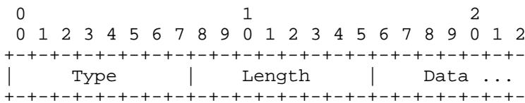
Figure 2: Type-Length-Value Extension Format for Mobile IPv4
