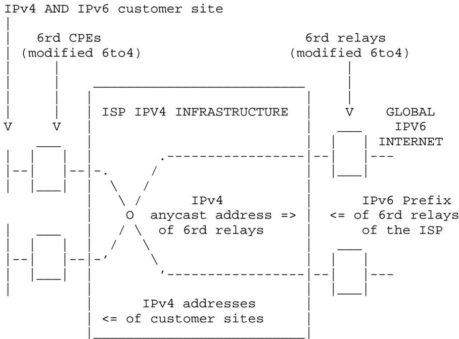
Figure 2: ISP Architecture to Deploy IPv6 with 6rd
