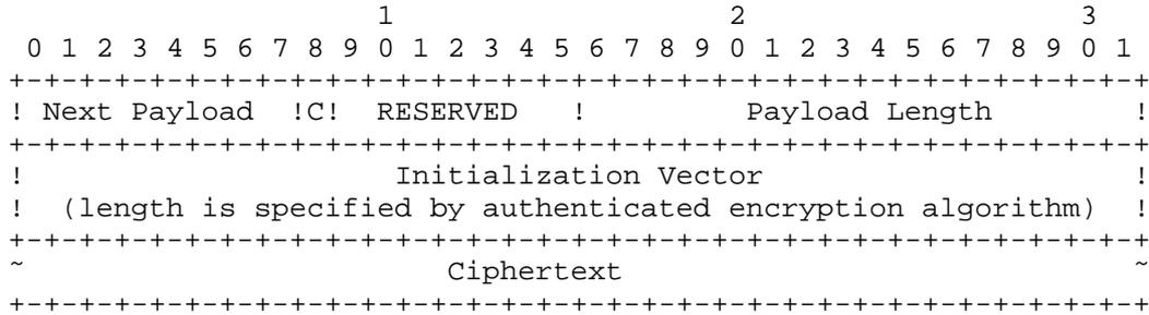
Figure 1. IKEv2 Encrypted Payload Data for Authenticated Encryption
