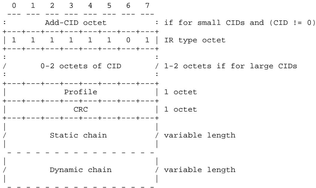
CRC: 8-bit CRC over the entire IR-header, including any CID fields and up until the end of the dynamic chain, using the polynomial defined in [RFC4995]. For purposes of computing the CRC, the CRC field is zero.
