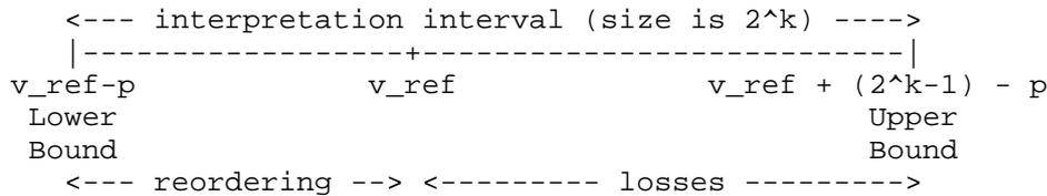
where  $p$  is the maximum negative delta, corresponding to the maximum reordering depth for which the lsb encoding can recover the original value of the field;
