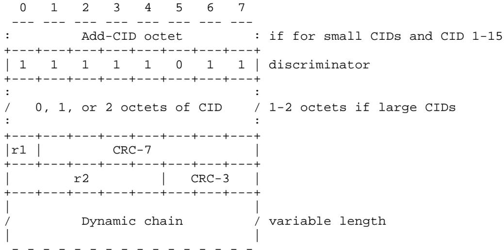
r1: MUST be set to zero; otherwise, the decompressor MUST discard the packet.
