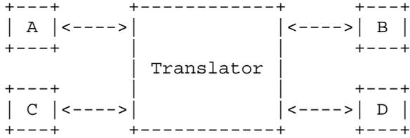
Figure 4 - RTP Translator (Relay) with Only Unicast Paths
