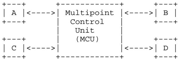
Figure 8 - Point to Multipoint Using Content Modifying MCUs
