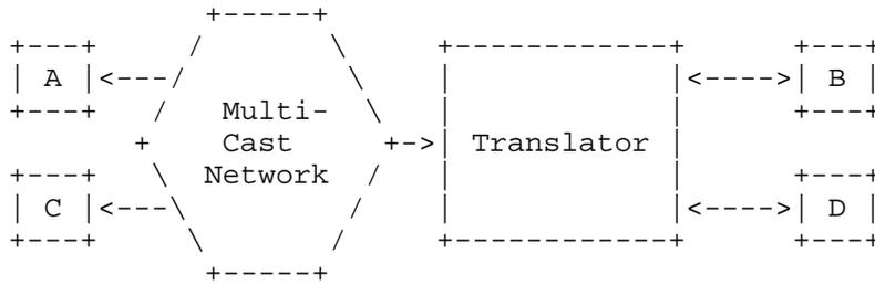
Figure 3 - Point to Multipoint Using a Translator
