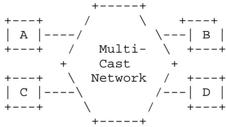
Figure 2 - Point to Multipoint Using Multicast
