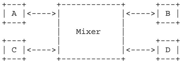
Figure 6 - RTP Mixer with Only Unicast Paths
