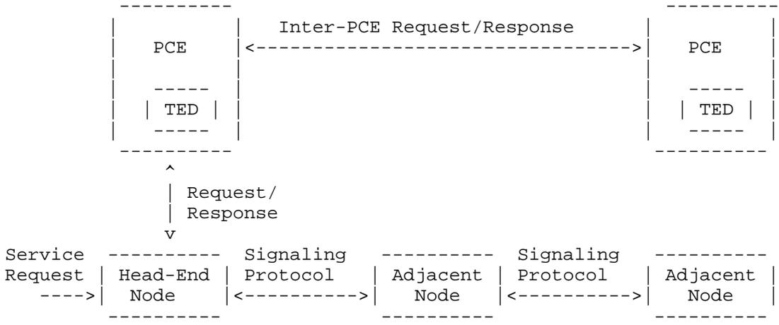
Figure 4. Multiple PCE Path Computation with Inter-PCE Communication
