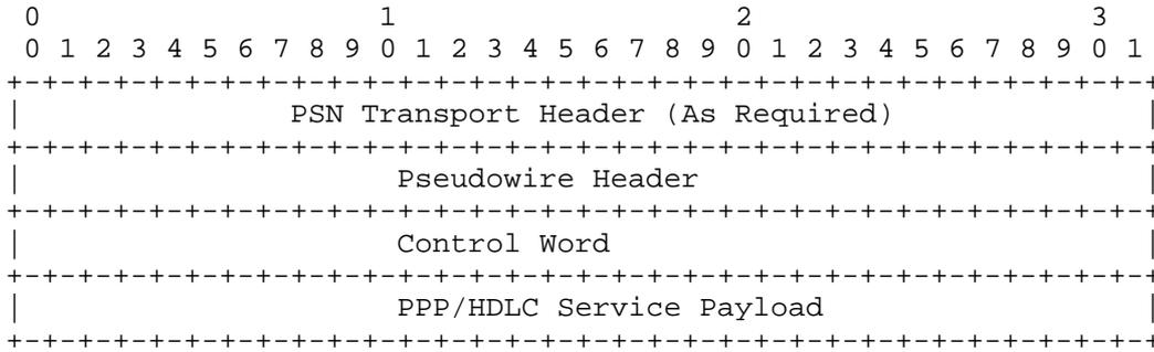
Figure 3. General format for PPP/HDLC encapsulation over PSNs
