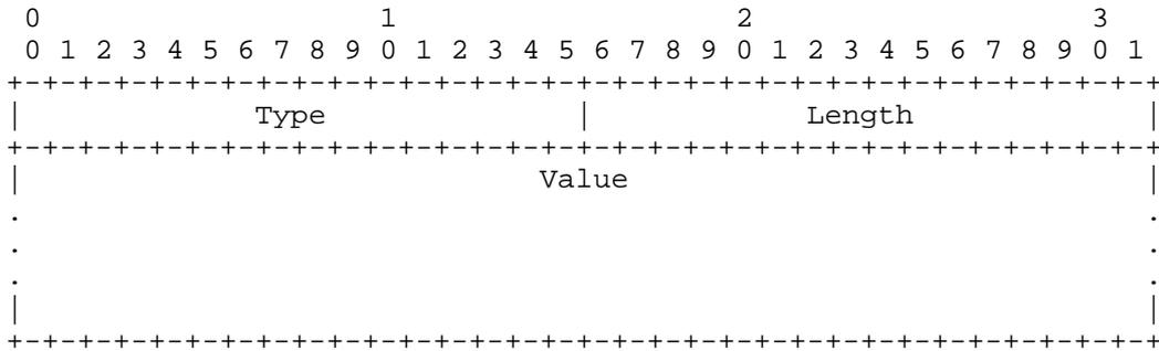
Types are defined below; Length is the length of the Value field in octets. The Value field depends on the Type; it is zero padded to align to a 4-octet boundary. TLVs may be nested within other TLVs, in which case the nested TLVs are called sub-TLVs. Sub-TLVs have independent types and MUST also be 4-octet aligned.
