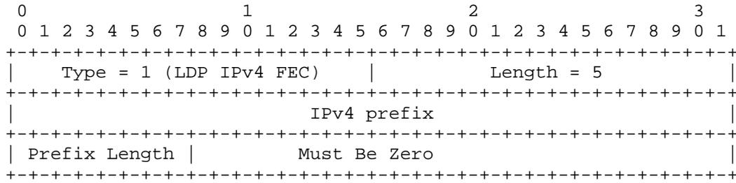
The Length for this TLV is 5. A Target FEC Stack TLV that contains an LDP IPv4 FEC sub-TLV and a VPN IPv4 prefix sub-TLV has the following format:
