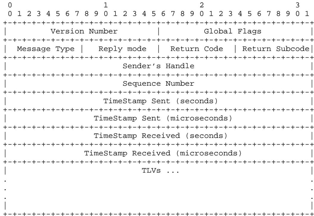
The Version Number is currently 1. (Note: the version number is to be incremented whenever a change is made that affects the ability of an implementation to correctly parse or process an MPLS echo request/reply. These changes include any syntactic or semantic changes made to any of the fixed fields, or to any Type-Length-Value (TLV) or sub-TLV assignment or format that is defined at a certain version number. The version number may not need to be changed if an optional TLV or sub-TLV is added.)
