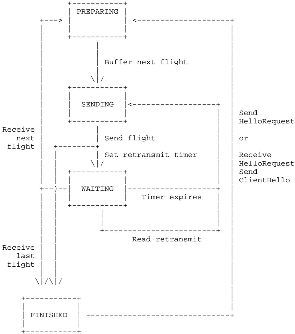
Figure 3. DTLS timeout and retransmission state machine
