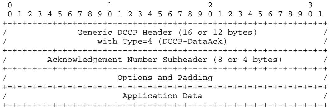
A DCCP-Data or DCCP-DataAck packet may have a zero-length application data area, which indicates that the application sent a zero-length datagram. This differs from DCCP-Request and DCCP-Response packets, where an empty application data area indicates the absence of
