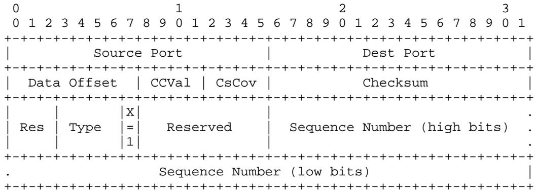
If X is zero, only the low 24 bits of the Sequence Number are transmitted, and the generic header is 12 bytes long.
