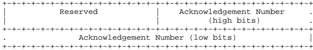
When X=0, only the low 24 bits of the Acknowledgement Number are transmitted, giving the Acknowledgement Number Subheader this format:
