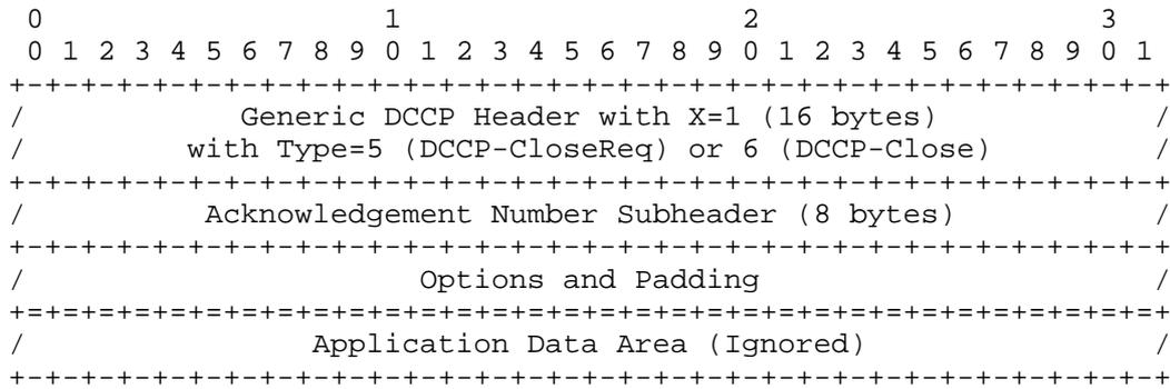
As with DCCP-Ack packets, DCCP-CloseReq and DCCP-Close packets MAY have non-zero-length application data areas, whose contents receivers MUST ignore.
