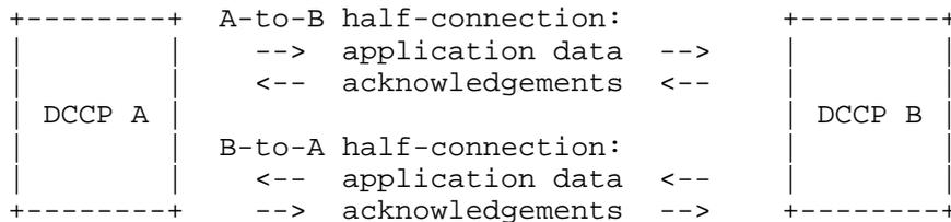
Although they are logically distinct, in practice the half-connections overlap; a DCCP-DataAck packet, for example, contains application data relevant to one half-connection and acknowledgement information relevant to the other.
