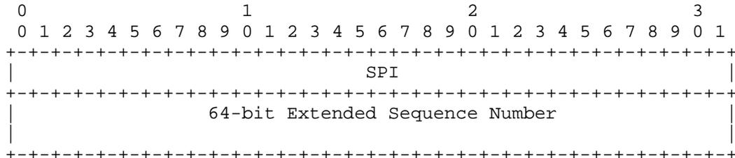
Figure 4. AAD Format with 64-bit Extended Sequence Number
