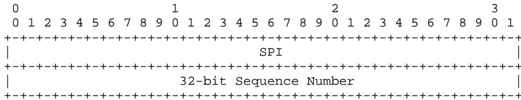
Figure 3. AAD Format with 32-bit Sequence Number
