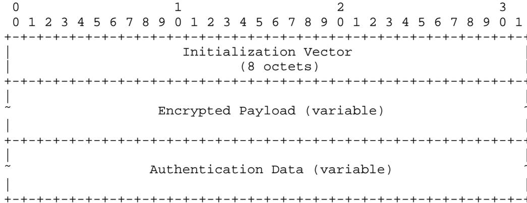
Figure 1. ESP Payload Encrypted with AES CCM
