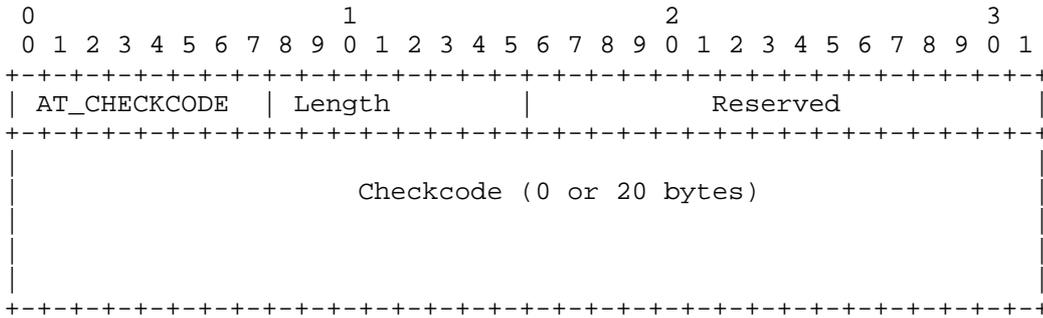
The value field of AT\_CHECKCODE begins with two reserved bytes, which may be followed by a 20-byte checkcode. If the checkcode is not included in AT\_CHECKCODE, then the attribute indicates that no EAP/-AKA-Identity messages were exchanged. This may occur in both full authentication and fast re-authentication. The reserved bytes are set to zero when sending and ignored on reception.
