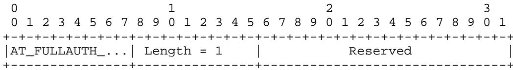
The use of the AT\_FULLAUTH\_ID\_REQ is defined in Section 4.1. The value field only contains two reserved bytes, which are set to zero on sending and ignored on reception.
