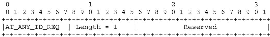
The use of the AT\_ANY\_ID\_REQ is defined in Section 4.1. The value field only contains two reserved bytes, which are set to zero on sending and ignored on reception.
