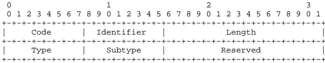
The rest of the Type-Data, immediately following the EAP-AKA header, consists of attributes that are encoded in Type, Length, Value format. The figure below shows the generic format of an attribute.
