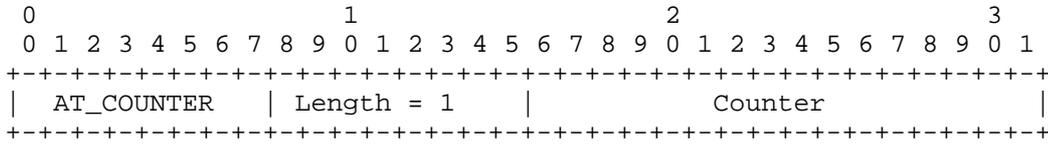
The value field of the AT\_COUNTER attribute consists of a 16-bit unsigned integer counter value, represented in network byte order. This attribute MUST always be encrypted by encapsulating it within the AT\_ENCR\_DATA attribute.
