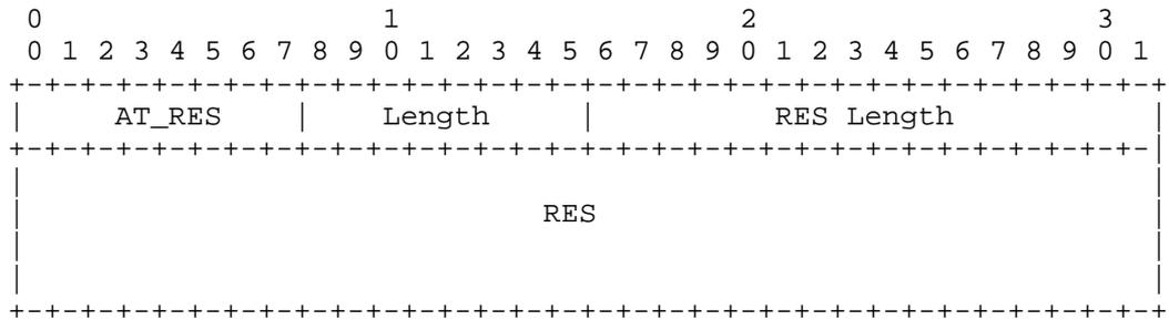
The value field of this attribute begins with the 2-byte RES Length, which identifies the exact length of the RES in bits. The RES length is followed by the AKA RES parameter. According to [TS33.105], the length of the AKA RES can vary between 32 and 128 bits. Because the length of the AT\_RES attribute must be a multiple of 4 bytes, the sender pads the RES with zero bits where necessary.
