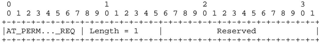
The use of the AT\_PERMANENT\_ID\_REQ is defined in Section 4.1. The value field only contains two reserved bytes, which are set to zero on sending and ignored on reception.
