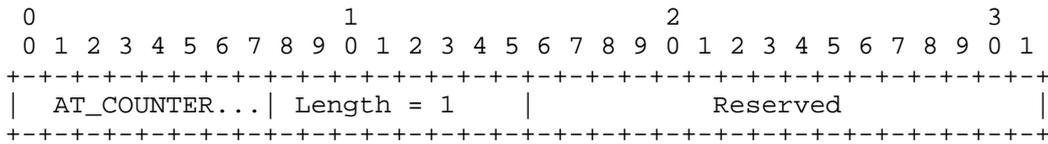
The value field of this attribute consists of two reserved bytes, which are set to zero upon sending and ignored upon reception. This attribute MUST always be encrypted by encapsulating it within the AT\_ENCR\_DATA attribute.
