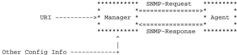
Additional configuration information (e.g., a security secret or key) may be provided via an interface other than that used for the URI. For example, when a managed device provides an SNMP URI in an unprotected fashion, that device should not provide a secret or key required to use the URI. The secret or key should instead be pre-configured in or pre-authorized to the manager; see Section 6.
