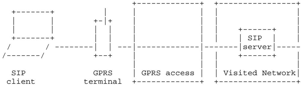
Figure 2: A computer connected to a GPRS terminal
