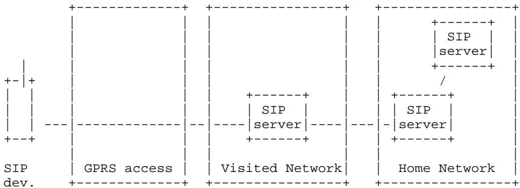
Figure 1: Overview of the 3GPP IMS architecture
