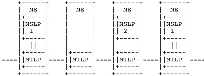
Figure 5: Signaling with Heterogeneous NSLPs
