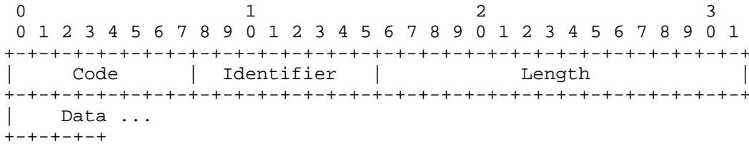
The Identifier and Length fields are as for LCP. The Code and Data fields and the processing of the messages are defined by the vendor-specific protocol.
