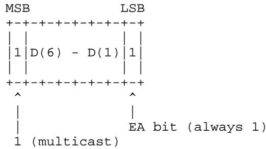
Figure 2. Address mapping in multicasting (MAPOS version 1).
