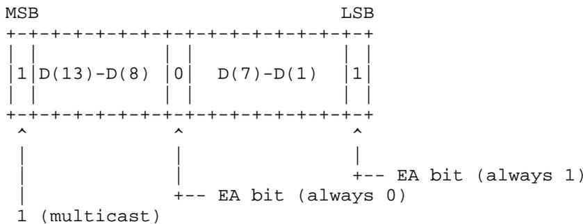
Figure 3. Address mapping in multicasting (MAPOS 16).
