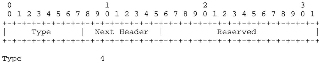
Next Header            Indicates the type of tunnelled data, using the same numbering as the IP Header Protocol Field.
