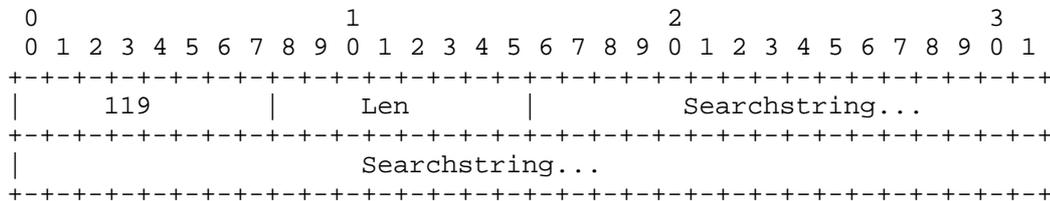
In the above diagram, Searchstring is a string specifying the searchlist. If the length of the searchlist exceeds the maximum permissible within a single option (255 octets), then multiple options MAY be used, as described in "Encoding Long Options in the Dynamic Host Configuration Protocol (DHCPv4)" [RFC3396].
