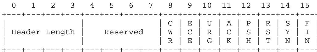
Figure 4: The new definition of bytes 13 and 14 of the TCP Header.
