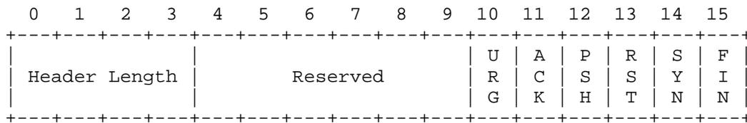
RFC 3168 defines two of the six bits from the Reserved field to be used for ECN, as follows:
