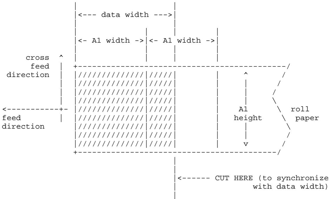
Example 2: "Auto-Cut", a device cutting the roll paper at multiples of fixed-size media width
