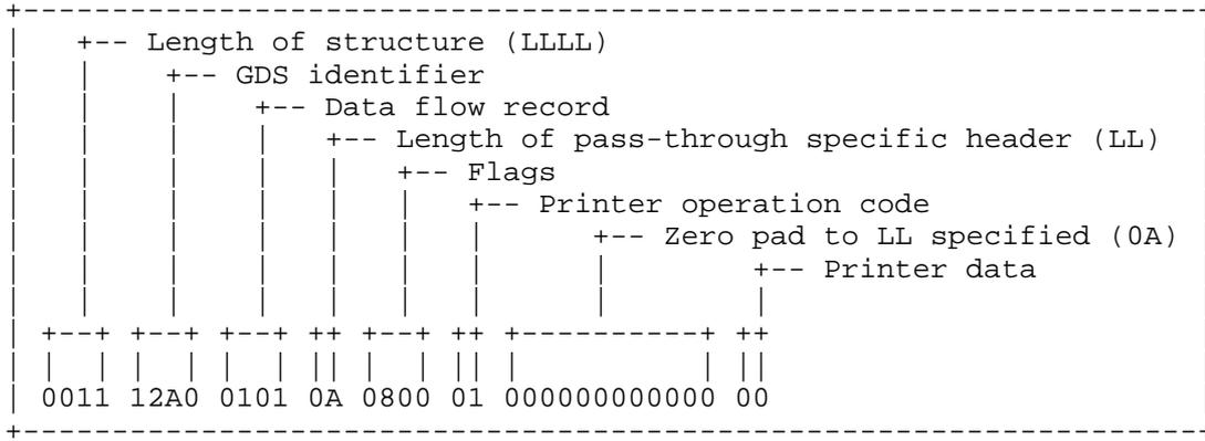
Figure 6. Server sending client a null print record
