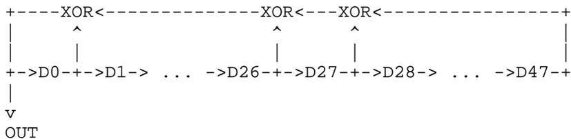
Each XOR is an exclusive-or gate; also known as a modulo-2 adder. Each  $D_n$  block is a D-type flip-flop clocked on the appropriate data clock.
