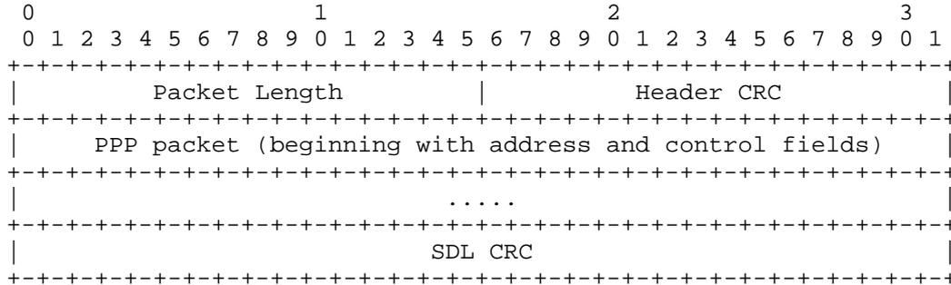
The four octet length header is DC balanced by exclusive-OR (also known as "modulo 2 addition") with the hex value B6AB31E0. This is the maximum transition, minimum sidelobe, Barker-like sequence of length 32. No other scrambling is done on the header itself.
