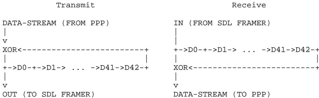
Each XOR is an exclusive-or gate; also known as a modulo-2 adder. Each Dn block is a D-type flip-flop clocked on the appropriate data clock.
