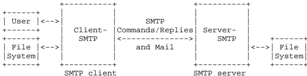
When an SMTP client has a message to transmit, it establishes a two-way transmission channel to an SMTP server. The responsibility of an SMTP client is to transfer mail messages to one or more SMTP servers, or report its failure to do so.
