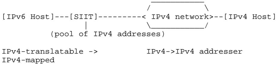
Figure 1. Using SIIT for a single IPv6-only subnet.
