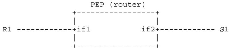
Figure 1: Unicast Example: a single PEP view
