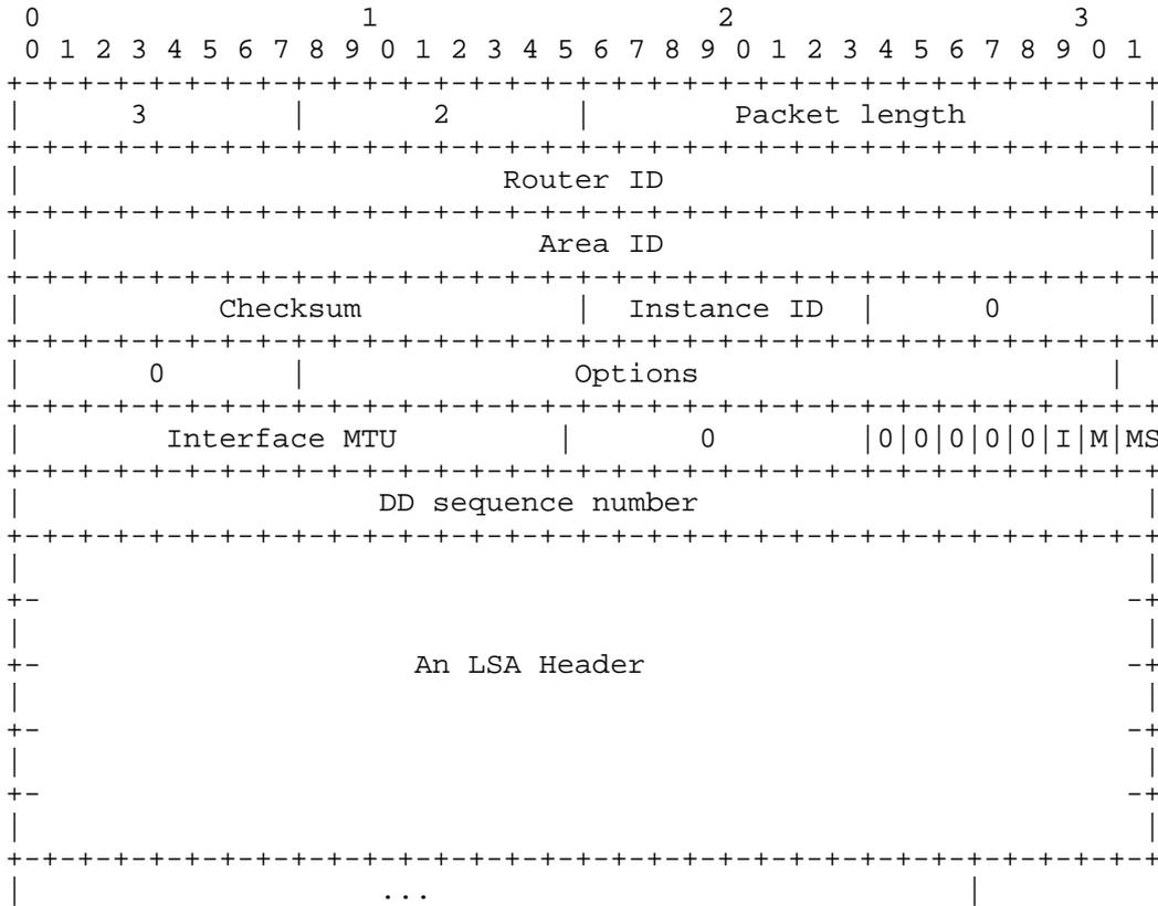
The format of the Database Description packet is very similar to both the Link State Request and Link State Acknowledgment packets. The main part of all three is a list of items, each item describing a piece of the link-state database. The sending of Database Description Packets is documented in Section 10.8 of [Ref1]. The reception of Database Description packets is documented in Section 10.6 of [Ref1].
