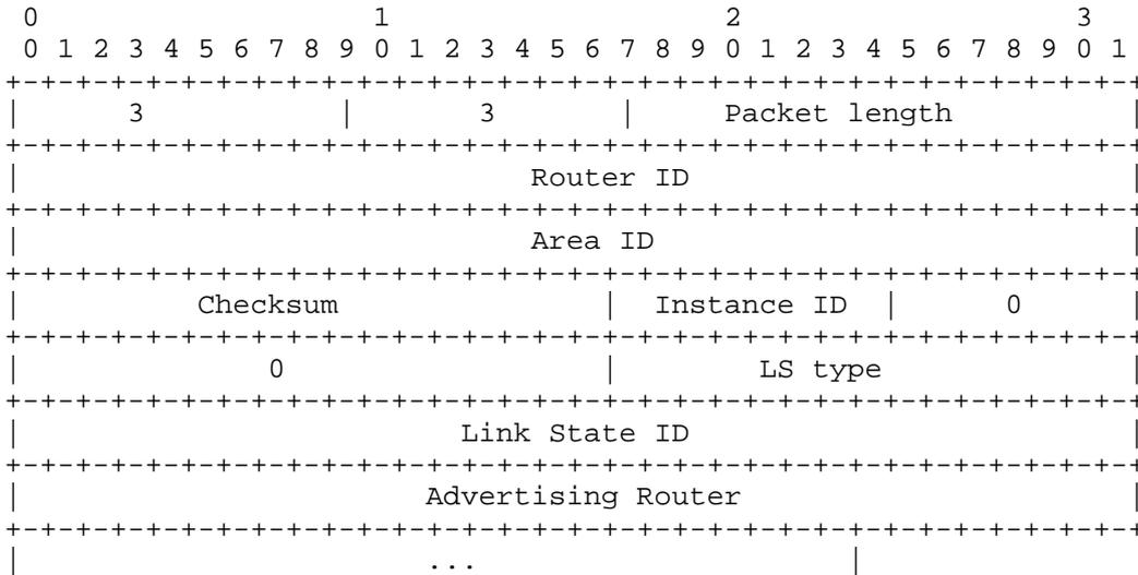
Each LSA requested is specified by its LS type, Link State ID, and Advertising Router. This uniquely identifies the LSA, but not its instance. Link State Request packets are understood to be requests for the most recent instance (whatever that might be).
