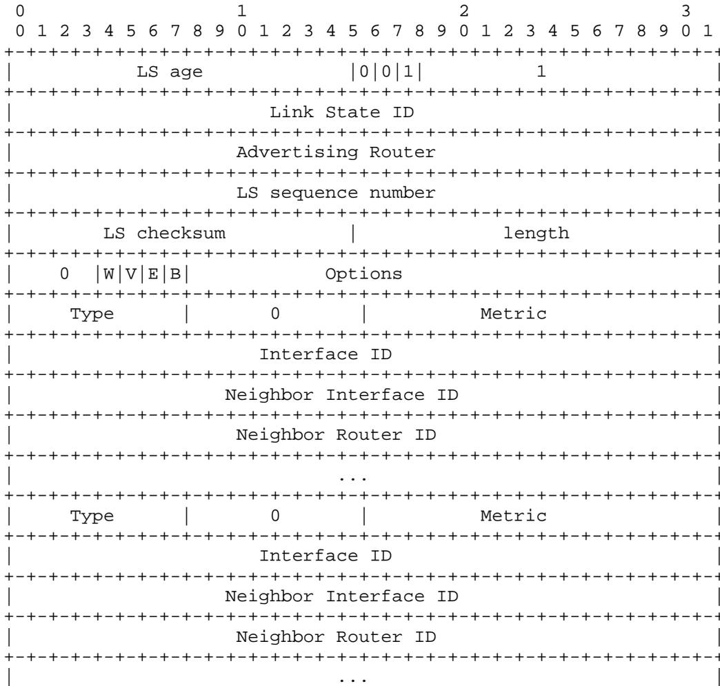
A single router may originate one or more Router LSAs, distinguished by their Link-State IDs (which are chosen arbitrarily by the originating router). The Options field and V, E and B bits should be the same in all Router LSAs from a single originator. However, in the case of a mismatch the values in the LSA with the lowest Link State ID take precedence. When more than one Router LSA is received from a single router, the links are processed as if concatenated into a single LSA.
