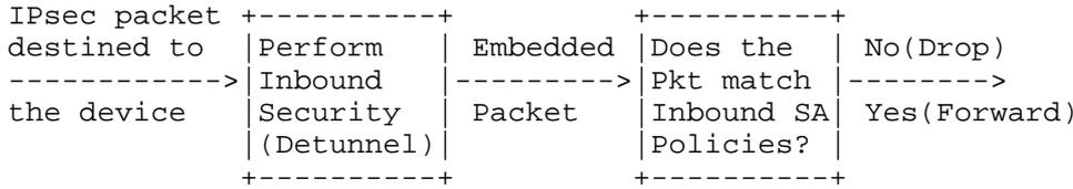
Figure 2. Operation of Tunnel-Mode IPsec on Incoming packets
