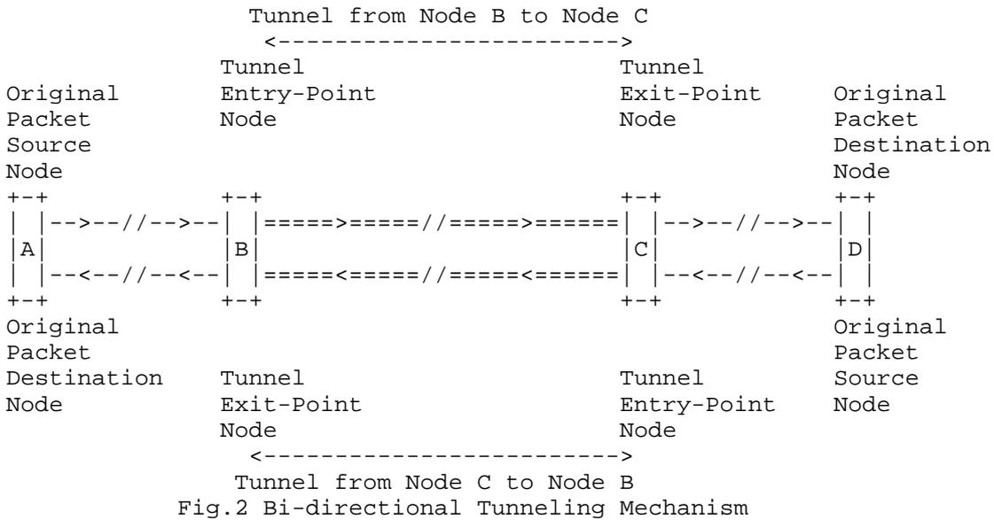
Fig.2 Bi-directional Tunneling Mechanism
