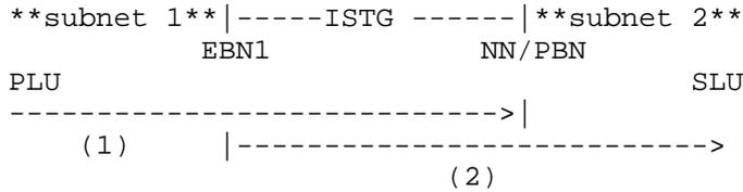
The value of the appnIsInRouteInfo object at EBN1 is the RSCV containing the route from the PLU (or the entry EBN in its subnet) to the NN or PBN, represented by (1). The value of the ebnIsRscvDestinationRoute object at EBN1 is the RSCV containing the route from EBN1 to the SLU, represented by (2). Note that the SLU must be in subnet 2, because the entry node is an NN or PBN rather than an EBN. The appnIsInRouteInfo object at NN/PBN contains the same RSCV, as represented by (2).
