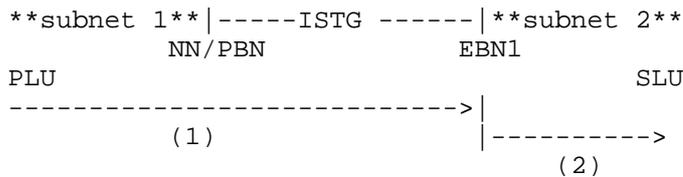
The value of the appnIsInRouteInfo object at the NN/PBN is the RSCV containing the route from the PLU to EBN1, represented by (1). Note that the PLU must be in subnet 1, because the exit node is an NN/PBN rather than an EBN. The appnIsInRouteInfo object at EBN1 contains the same RSCV. The value of the ebnIsRscvDestinationRoute object at EBN1 is the RSCV containing the route from EBN1 to the SLU (or the next subnet's entry border node), as represented by (2).
