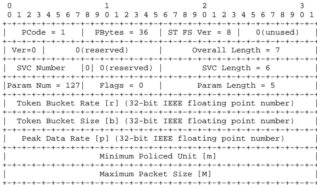
Fig. 3.1: Format of ST FlowSpec for Controlled-Load Service.
