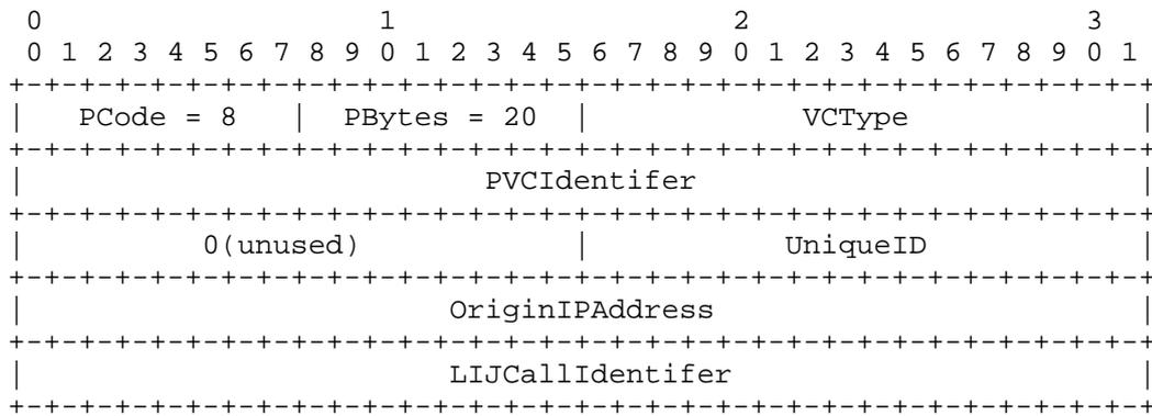
Fig. 3.2: Format of VC-type common SCMP element.
