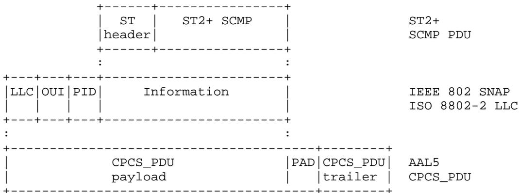
Fig. 6.2: RFC 1483 base encapsulation.
