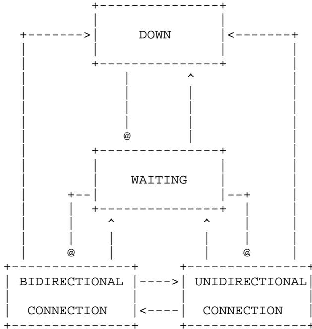
Figure 1: Hello Finite State Machine (HFSM)
