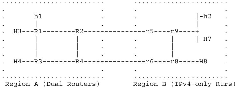
Figure 2: Example of Automatic Tunneling
