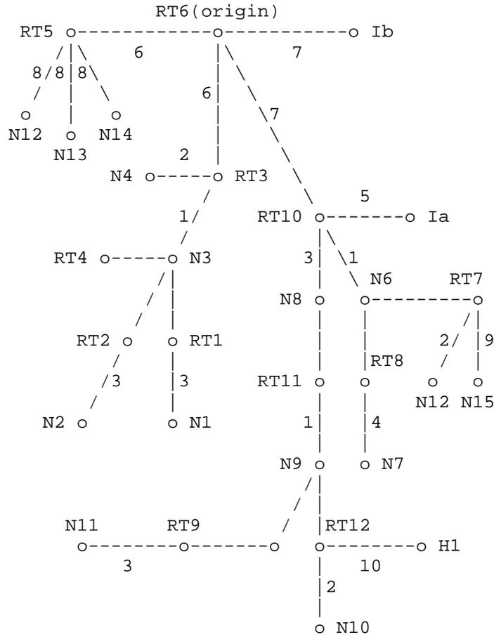
Figure 5: The SPF tree for Router RT6
