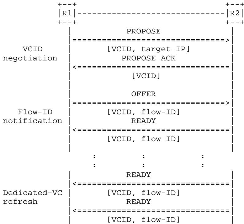
Figure 2. Flow ID notification and refresh procedure
