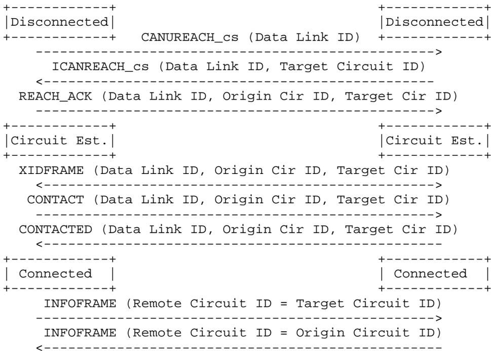
During the exchange of the XIDFRAME, CONTACT, and CONTACTED messages, the pair of Circuit ID parameters is included in the message format along with the DATA LINK ID parameter. Once the connection has been
