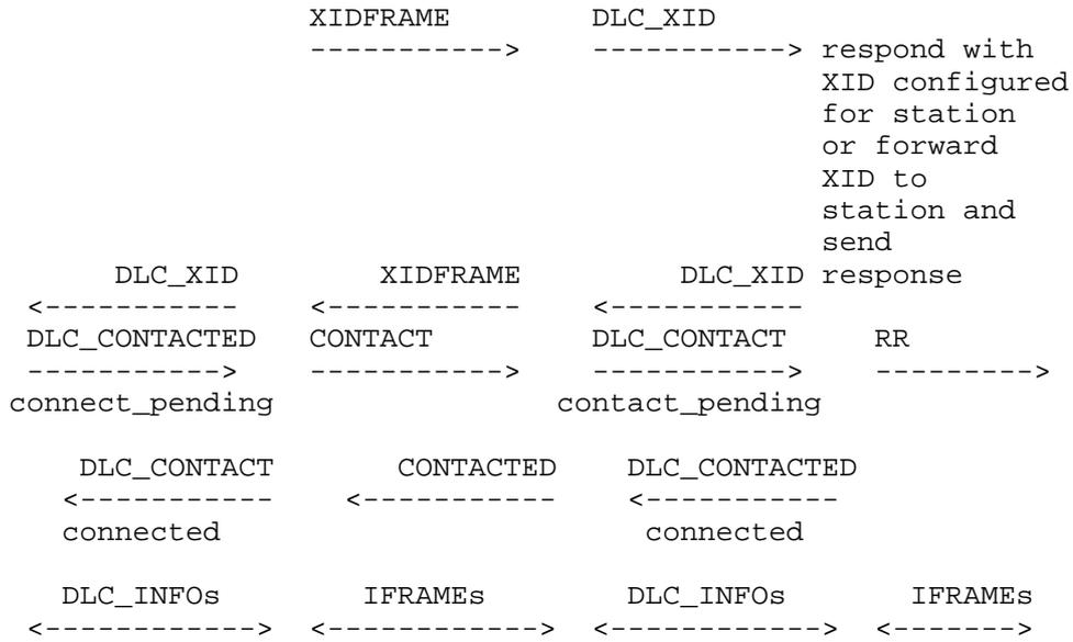
Here is an example of a switched SDLC PU 2.0 device as the target station.
