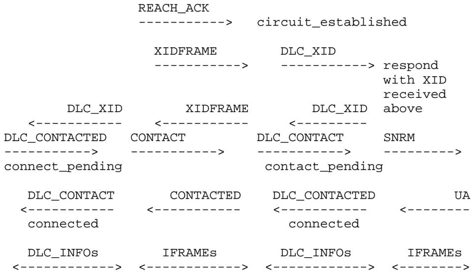
Here is an example of an SDLC T2.1 device as the target station.
