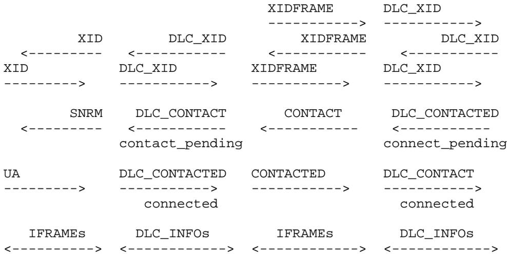
Here is an example of a leased SDLC PU 2.0 device as the target station.
