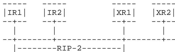
The Internal Routers (IR1 and IR2) are only running RIP-2. The External Routers (XR1 and XR2) are both running BGP, for example; however, only XR1 is running BGP and RIP-2. Since XR2 is not running RIP-2, the IRs will not know of its existence and will never use it
